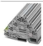
Motor terminal block, four-level, with PE foot, connection method: spring-cage connection, cross section: 0.08 mm² - 4 mm², AWG: 28 - 12, width: 5.2 mm, color: gray, mounting type: NS 35/7,5, NS 35/15
