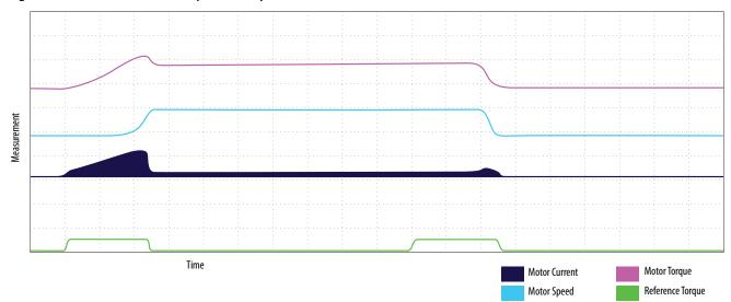
Figure 51 - Soft Start and Soft Stop on Conveyor
