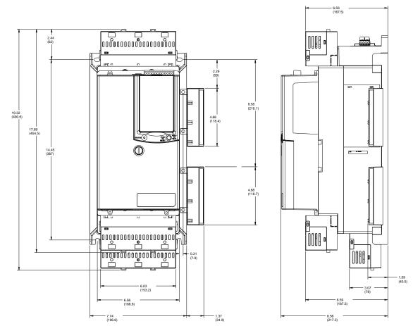
Figure 24 - 108/135 A Controller with Internal Bypass: With Terminal Covers and MOV Options
