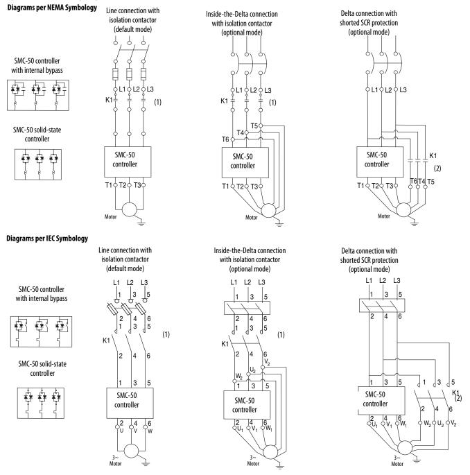
(1) Contactor must be fully rated for motor Hp/kW and FLA.
