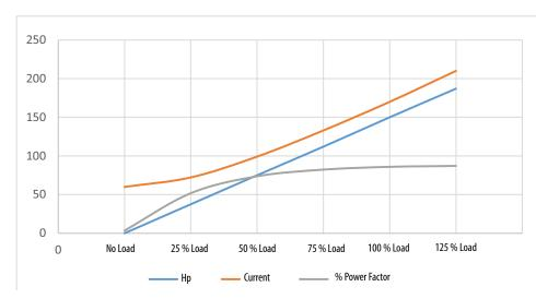
Figure 50 - Pump Cavitation and Blockage (for 150 Hp Motor)
