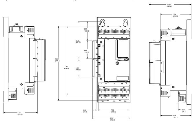
Note: When mounted in an enclosure, maintain a minimum of 6.0 inches (152.4 mm) clearance above and below the SMC-50 controller. Side-to-side clearance is not required.
