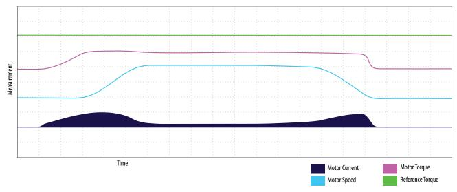
These two scenarios use identical motors and starting parameters. Note the difference between the two starts. The sensorless linear acceleration provides smoother motor torque over the soft starting method. Unlike soft start, which is load dependent, linear acceleration can produce a more accurate starting time. Sensorless linear acceleration also produces a smoother motor current, torque, and speed.
