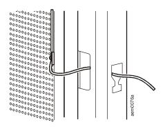
8. Route the cords between the vertical support rail and the side panel. Each 13-ft (4-m) sensor cord may be extended to a maximum of 50 ft (15 m), using RJ-45 couplings and standard CAT5 cables.
