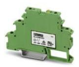
Relay terminal block, with soldered-in miniature power relay, contacts (AgSnO): medium to large loads, 1 PDT, input voltage 24 V DC, for assembly on NS 35/7.5, terminal width 6.2 mm
