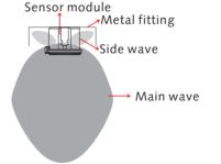
Microwave detection includes two parts called main wave and side wave. Main wave normally detects the motion signal. Side wave does not effect motion detection but might disturb main wave if the microwave motion sensor is built-in a sealed metal luminaire as microwave can not pass through metal.
