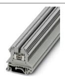
Feed-through terminal block, Connection method: Screw connection, Cross section: 0.14 mm² - 1.5 mm², AWG: 26 - 16, Width: 4.2 mm, Color: gray, Mounting type: NS 35/7,5, NS 35/15, NS 32
