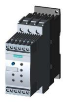
SIRIUS soft starter S0 25 A, 15 kW/500 V, 40  $^{\circ}\text{C}$  400-600 V AC, 24 V AC/DC Screw terminals Thermistor motor protection
