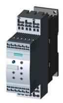
SIRIUS soft starter S0 25 A, 11 kW/400 V, 40  $^{\circ}\text{C}$  200-480 V AC, 24 V AC/DC spring-type terminals Thermistor motor protection
