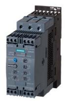
SIRIUS soft starter S2 72 A, 37 kW/400 V, 40  $^{\circ}\text{C}$  200-480 V AC, 110-230 V AC/DC Screw terminals
