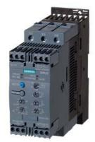
SIRIUS soft starter S2 72 A, 45 kW/500 V, 40  $^{\circ}\text{C}$  400-600 V AC, 24 V AC/DC Screw terminals Thermistor motor protection
