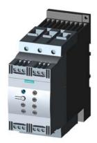
SIRIUS soft starter S3 80 A, 45 kW/400 V, 40  $^{\circ}\text{C}$  200-480 V AC, 24 V AC/DC Screw terminals Thermistor motor protection
