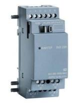
SIPLUS LOGO! DM8 230 V -40...+70°C start up -25°C with conformal coating based on 6ED1055-1FB00-0BA2 . Expansion module, PS/I/O: 230V/230V/relay, 2 MW, 4 DI/4 DO for LOGO! 8
