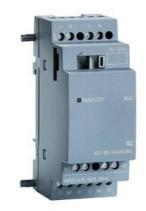
SIPLUS LOGO! AM2 -40...+70°C start up -25°C with conformal coating based on 6ED1055-1MA00-0BA2 . Expansion module, PS/: 12/24 V DC, 2 AI, 0-10 V or 0/4-20 mA for LOGO! 8
