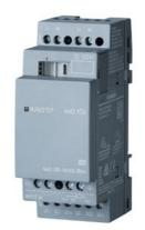
SIPLUS LOGO! AM2 RTD -40 ... 70°C start up -25°C with conformal coating based on 6ED1055-1MD00-0BA2 . extens. module, PS: 12/24 V DC, 2AI-50...+200°C Pt100/1000 for LOGO! 8
