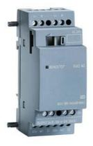
SIPLUS LOGO! AM2 AQ -40...+70 °C start up -25°C with conformal coating based on 6ED1055-1MM00-0BA2 . Expansion module, PS: 24 V DC, 2 AO, 0-10 V, 0/4-20 mA for LOGO! 8
