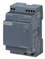
SIPLUS LOGO! Power 24 V 2.5 A for exposure to environmental substances -40...+70 °C start up at -25 °C based on 6EP3332-6SB00-0AY0 . stabilized power supply input: 100-240 V AC output: 24 V DC/ 2.5 A
