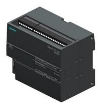
SIMATIC S7-200 SMART, CPU CR40, compact CPU, AC/DC/relay, onboard I/O: 24 DI 24 V DC; 16 DO relay 2A; Power supply: AC 85-264 V AC at 47-63 Hz, Program/data memory 20 KB
