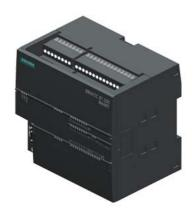
\*\*\* spare part \*\*\* SIMATIC S7-200 SMART, CPU SR30, standard CPU, AC/DC/relay, onboard I/O: 18 DI 24 V DC; 12 DO relay 2 A; power supply: AC 85-264 V AC at 47-63 Hz, program/data memory 30 KB
