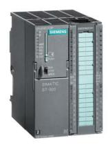
SIMATIC S7-300, CPU 313C-2 DP Compact CPU with MPI, 16 DI/16 DO, 3 high-speed counters (30 kHz), integrated DP interface, Integr. power supply 24 V DC, work memory 128 KB, Front connector (1x 40-pole) and Micro Memory Card required
