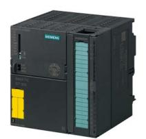
SIMATIC S7-300, CPU 317TF-3 PN/DP, Central processing unit for PLC, Technology and safety tasks, 1.5 MB work memory, 1st interface MPI/DP 12 Mbit/s, 2nd interface DP (drive), 3rd interface Ethernet PROFINET with 2-port switch, Integr. I/O for technology, Front connector (1x 40-pole) and Micro Memory Card min. 8 MB required
