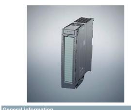
SIMATIC S7-1500, digital output module DQ 16x 230V AC/2A ST; relay 16 channels in groups of 2; 4 A per group; switching cycle counter for integrated relay, diagnostics; substitute value: the module supports the safety-oriented shutdown of load groups up to SIL1 according to EN IEC 62061:2021 and Category 2 / PL c according to EN ISO 13849-1:2015. front connector (screw terminals or push-in) to be ordered separately
