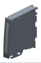
SIMATIC S7-1500, analog output module AQ 2x U/I ST, 16-bit resolution accuracy 0.3%. 2 channels in groups of 2, diagnostics; substitute value; the module supports the safety-oriented shutdown of load groups up to SIL2 according to EN IEC 62061:2021 and Category 2 / PL c according to EN ISO 13849-1:2015. delivery including front connector push-in, infeed element, shielding bracket and shield terminal
