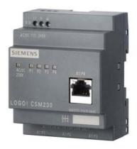
LOGO! CSM 230 Compact Switch Module of connection of a LOGO! (... 0BA7) and up to 3 further nodes to Industrial Ethernet with 10/100 Mbit/s; unmanaged switch, 4 RJ45 ports, 1x front port for diagnostics AC/DC 115 ... 240 V
