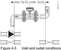
Figure 4-5 Thiet and Outlet Conditions
