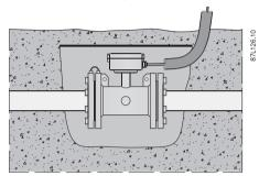
Figure 5-2 Direct burial of sensor
