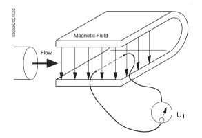
$U_i$  = When an electrical conductor of length L is moved at velocity v, perpendicular to the lines of flux through a magnetic field of strength B, the voltage  $U_i$  is induced at the ends of the conductor
