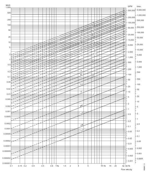
The tables show the relationship between flow velocity v, flow quantity Q and sensor dimension DN.
