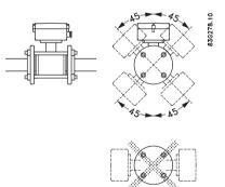
Figure 4-7 Horizontal installation, various terminal box positions
