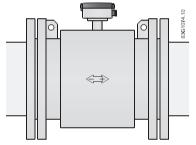
Figure 4-8 Potential equalization with earthing electrodes
