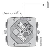
4. Fit the  $\frac{1}{2}$ " NPT or M20 cable glands for supply and output cables.
