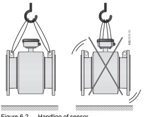
Figure 6-2 Handling of sensor
