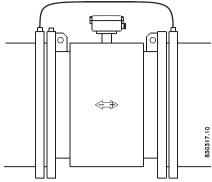
Figure 4-9 Cathodic protection
