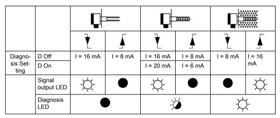
The output current can indicate weak vibration amplitude with the diagnosis setting **D ON**. If the diagnosis is set to **D OFF**, the output will be either 8 mA or 16 mA depending on high or low level settings.
