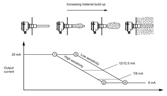
Vibration damping by material
