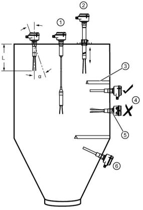
Position tines vertically to avoid product buildup: use a 50 mm open-end wrench to turn the process connection until the tine orientation marking faces up or down.
