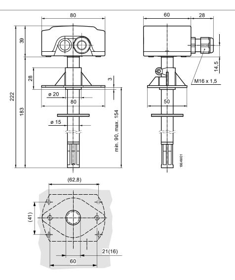
Drilling plan with (without) mounting flange
