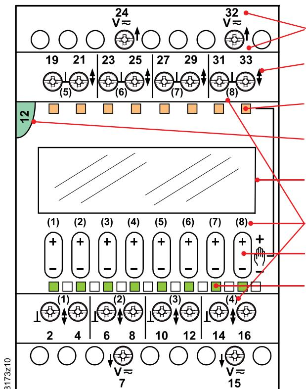
Connection terminals (No. 1 screwdriver for slotted or recessed-head \* screws)
