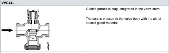
Caution: The 2-port seat valve does not become a three-port valve by removing the cover plate!
