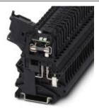
Fuse modular terminal block, fuse type: Glass / ceramics / ..., connection method: Screw connection, cross section: 0.14 mm²- 6 mm², AWG: 26 - 10, nominal current: 6.3 A, nom. voltage: 500 V, width: 6.2 mm, fuse type: G / 5 x 20, mounting type: NS 35/7,5, NS 35/15, color: black
