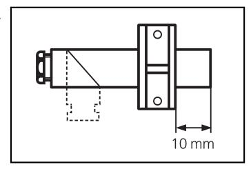
Open space around the sensing face when mounted in metal:
