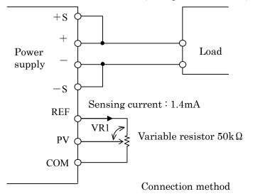
When output voltage is over rated value, please make sure that maximum output power is below rated value. Moreover, when output voltage is below rated value, please make sure that maximum output current is below rated value.
