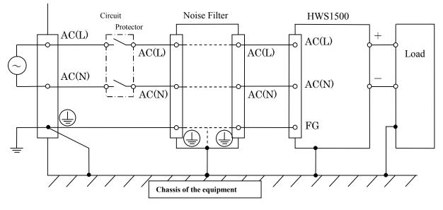
Recommended circuit protector : AC250V30A Recommended noise filter : MXB1220 (DENSEI-LAMBDA) (8) M4 screw for output terminal might damage the terminal's inner thread. This is mainly cause by the M4 screw's unthread section. Therefore, please select a washer, spring washer, etc. to avoid unthread screw section from penetrating into output terminal inner section.
