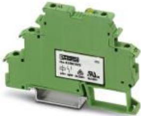
Relay terminal block, with soldered-in miniature power relay, contacts (AgSnO): medium to large loads, 1 PDT, input voltage 24 V DC, for assembly on NS 35/7.5, terminal width 6.2 mm
