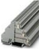
Sensor/actuator terminal block, connection method: Screw connection, cross section: 0.2 mm<sup>2</sup> - 4 mm<sup>2</sup>, AWG: 24 - 12, width: 6.2 mm, color: gray, mounting type: NS 35/7,5, NS 35/15
