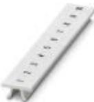
Zack marker strip, Strip, white, labeled, can be labeled with: CMS-P1-PLOTTER, printed horizontally: consecutive numbers 1 ... 10, 11 ... 20, etc. up to 491 ... 500, mounting type: snap into tall marker groove, for terminal block width: 6.2 mm, lettering field size: 6.15 x 10.5 mm, Number of individual labels: 10
