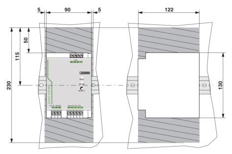
Slim-style installation: Installation depth 125 mm (+ DIN rail) (state at delivery)
