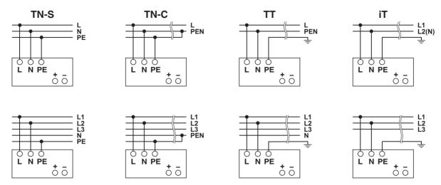
The connection for 100 V AC ... 240 V AC is established using the L, N, and P screw connections.
