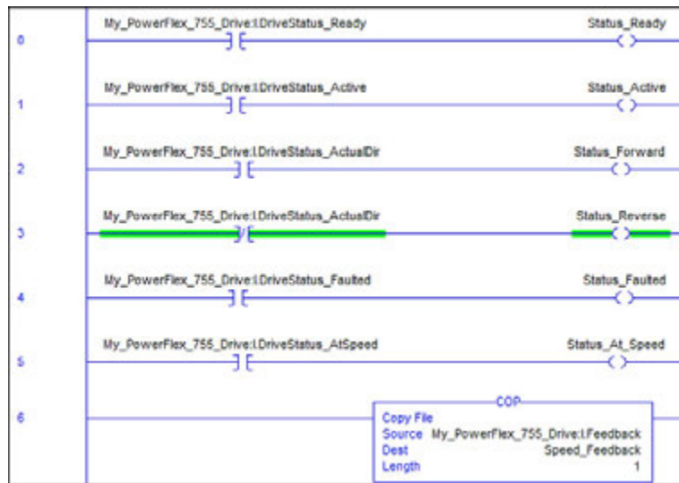
Figure 25 - ControlLogix Controller Example Ladder Logic Program Using a Drive Add-on Profile for Logic Command/Reference
