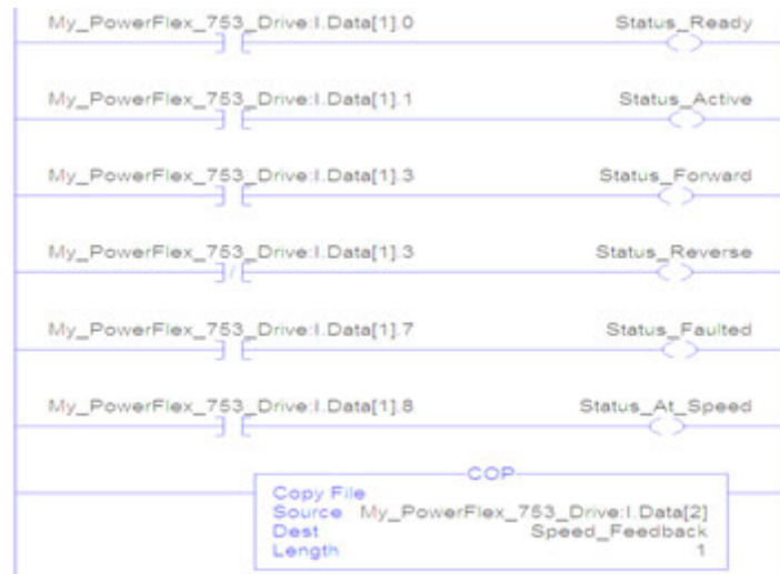
Figure 28 - ControlLogix Controller Example Ladder Logic Program Using a Drive Generic Profile for Logic Status/Feedback
