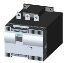
SIRIUS soft starter Values at 400 V, 40 °C standard: 313 A, 160 kW Inside-delta: 542 A, 315 kW 200-460 V AC, 230 V AC Screw terminals !!! Phased-out product !!! Successor is SIRIUS 3RW5, Preferred successor type is >>3RW5545-6HA14<<
