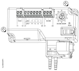
IP54 box mounting: The IP54 rated APS can only be mounted as shown.
