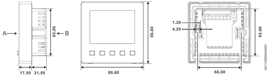
Above are the dimensions for the thermostat and its mounting plate.
